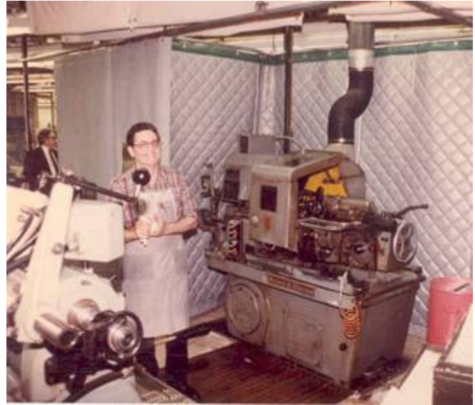
Typical BAC-110R HUSH FLEX™ curtain system (ceiling suspended) around a screw machine. Features include double track sliding panel access, viewing windows and overhead baffles.
