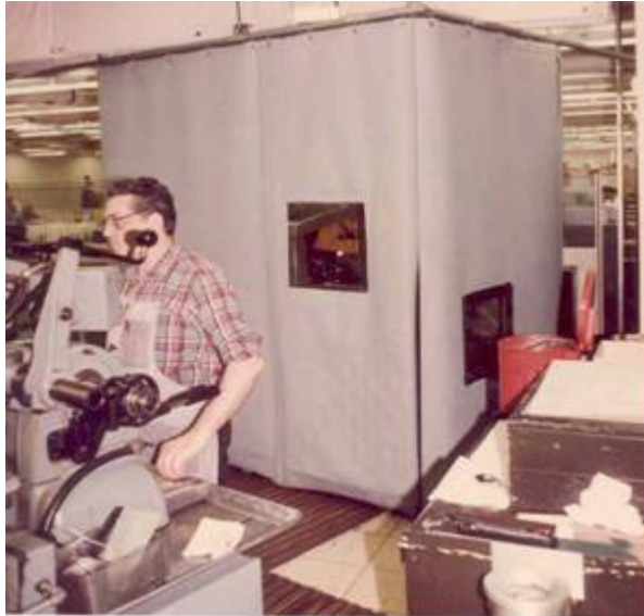
Typical BAC-110R HUSH FLEX™ curtain system (ceiling suspended) around a screw machine. Features include double track sliding panel access, viewing windows and overhead baffles.
