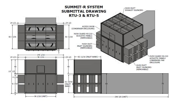
BRD Noise & Vibration Control, Inc. designed, manufactured and installed these Hushcore® Summit-R™ model HDE-2I2E System consisting of 2′ intake silencers and 2′ fan discharge stack sections to provide turn-key noise solutions for all (7) units.
