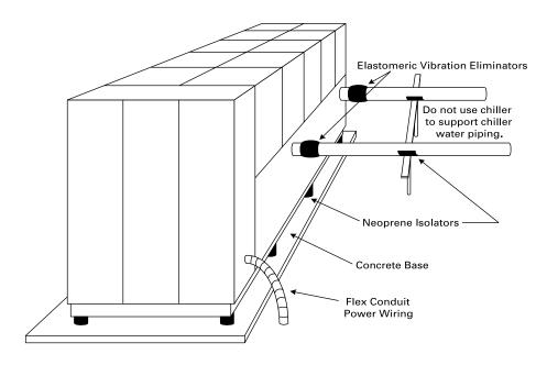
within the spring. Elastomeric isolation or neoprene isolators, however, were determined to be up to 90 percent effective when subjected to the same test. Neoprene isolators have the ability to not only dampen, but also to absorb, the vibration created by the screw compressor. This eliminates any unnecessary noise transmission throughout the building in addition to protecting the chiller and surrounding components.
