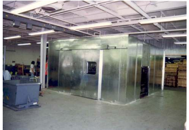
Type HG-400 panels are used to quiet an Amada automatic punch press. Design features include sliding access doors for material flow and integration of the control panel in the right side of the enclosure.
