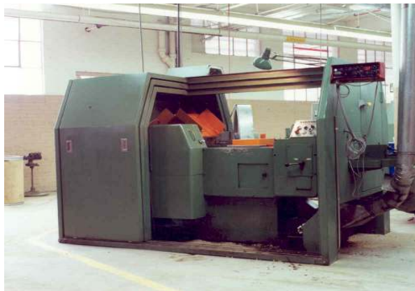
Header equipment enclosure with telescoping HGNP-201 access doors.
