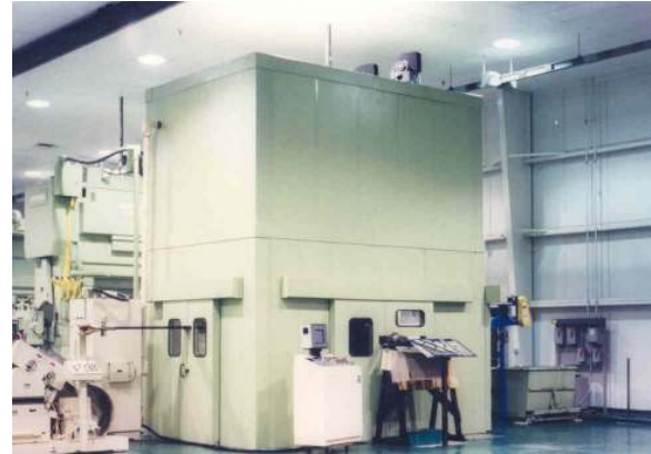
Minster punch press enclosure using type HG-400 panels.
