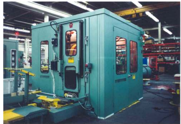
Custom OEM machinery enclosure with pneumatically operated access door.
