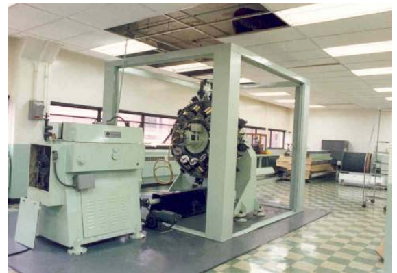
HUSH GUARD™ type SE enclosure with side wall panels removed.
