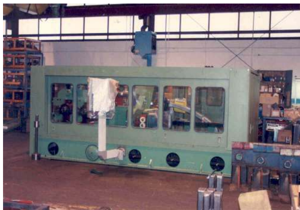
HGNP-402 enclosure with lift-out sliding access doors forming machine tool.
